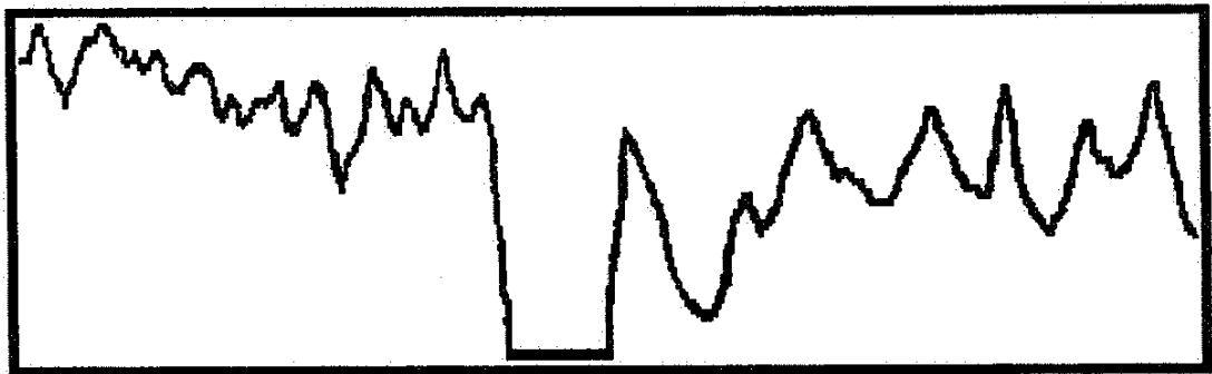
PROFILE DETAIL REVEALED BY RESTRICTING STYLUS MOVEMENT INTO SURFACE INTERRUPTION (I.E. DEEP SCRATCH).
